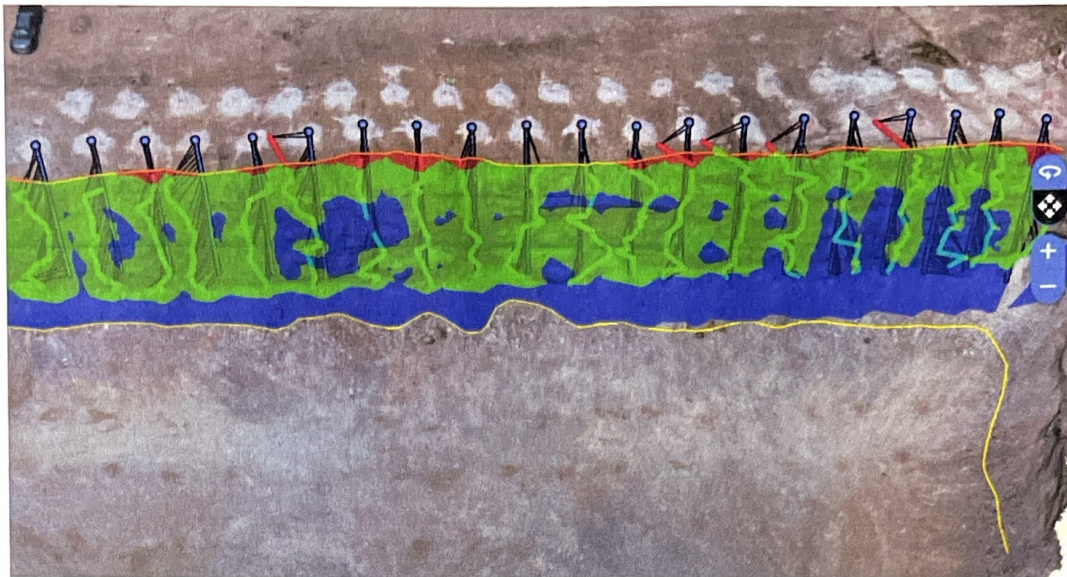
Aerial view of blast pattern created from 3D profile software
