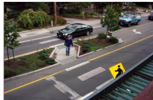
Crossing islands provide refuge for people crossing the street and enable them to cross a single direction of traffic at a time.
